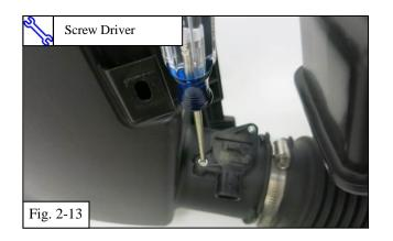
(m) Undo the MAFS screws and remove the MAFS from the factory airbox lid, retain for later use. (Fig 2-13)
