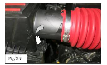
(i) Make sure the two (2) tabs on the Airbox lid and Lower housing are fully engaged.
